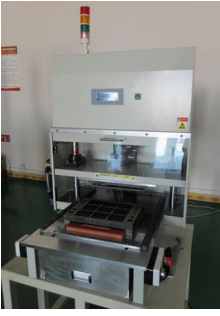
Punching type PCB cutter machine for cutting the complex PCB board
