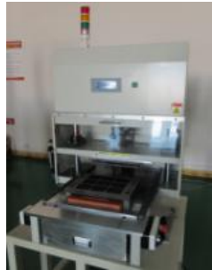
Note:Punching type PCB cutter machine for cutting the complex PCB board
